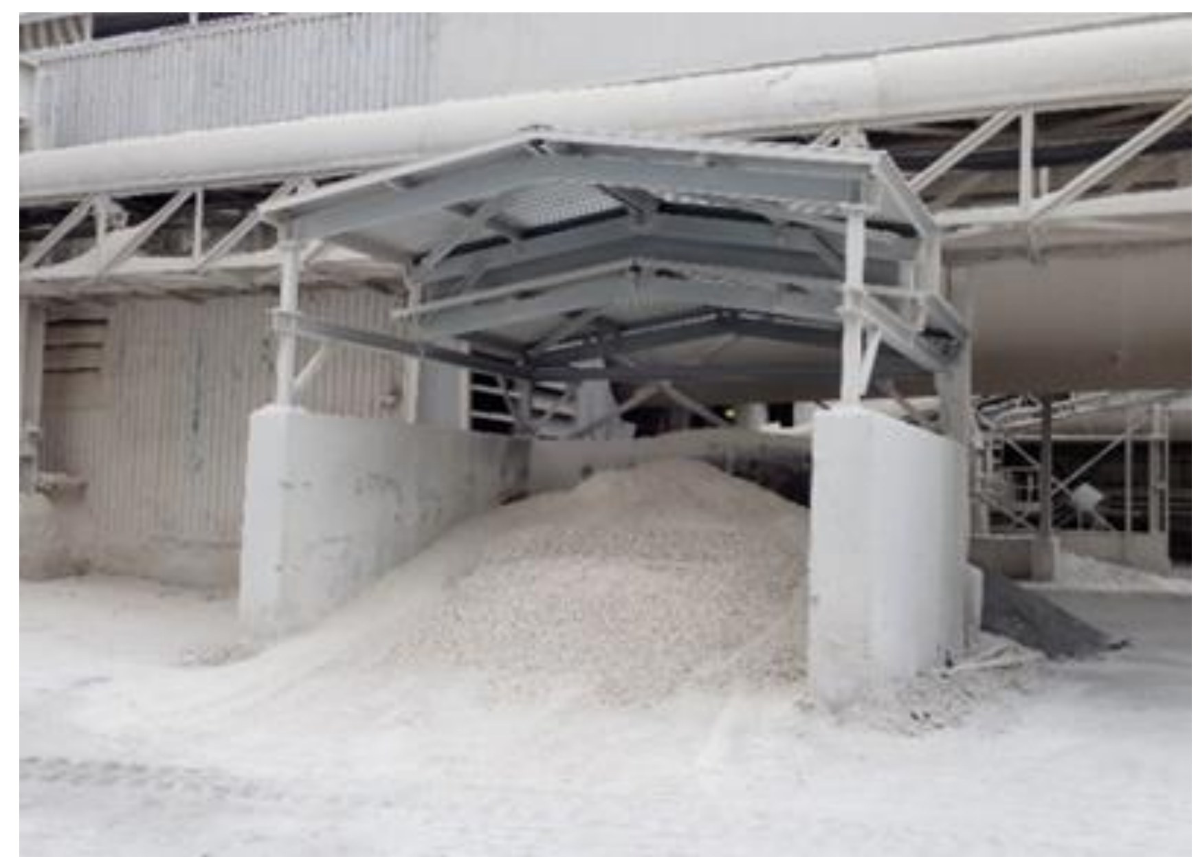
December 2018: Short-term storage of a small quantity of lime in a designated enclosure
