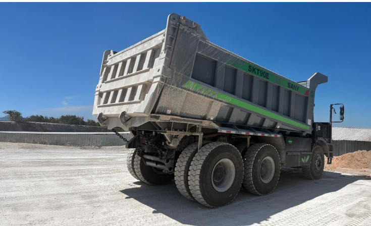
Rechargeable electric trucks at the Soma quarry in Turkey
